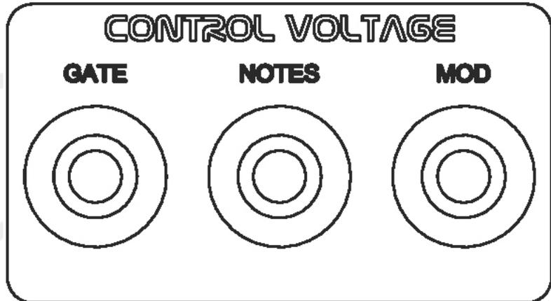
Using the jumpers on the circuit board, the sockets can also be configured as inputs. The SYNTHLAB can then be controlled through the GATE, NOTES-CV and MOD-CV. (The internal MIDI interface is then switched off).
