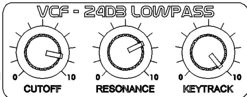
From a musical point of view, the low pass is easily the most productive filter. The low pass allows all frequencies below the so called frequency limit to pass through, cutting off frequencies above the limit. The frequency limit is adjusted using the CUT-OFF control.
