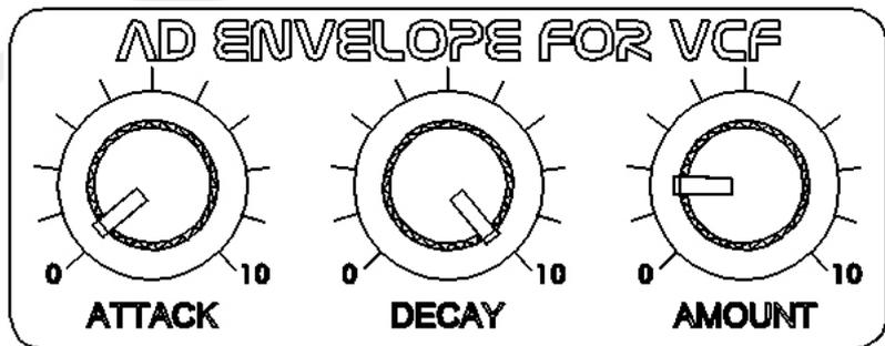
envelope, which is not so important. As we do not possess the hearing to detect slight changes in frequency (as opposed to changes in volume), the VCF envelope curve is therefore in synthesisers generally not as complex as the volume envelope curve. Using the AMOUNT adjustment, the effect of the envelope curve on the filter frequency can be set.
