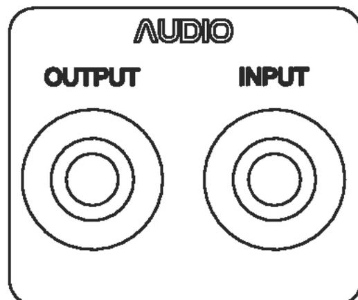
The sockets are 6.3mm jack sockets (mono), making possible a simple integration of the unit with professional studio equipment.
